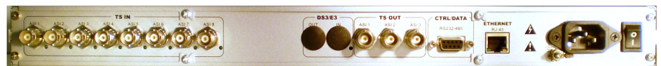
8-input back panel with ASI Interface (note option for DS3/E3 out/in connectors)
